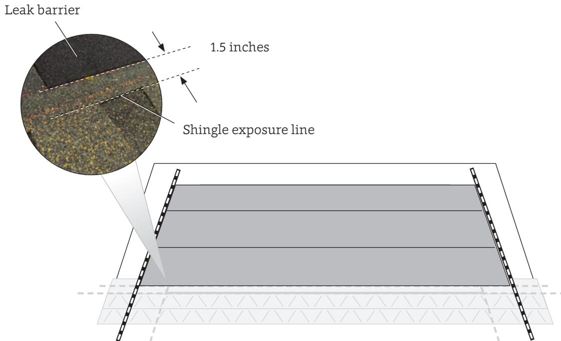
**Figure 20. Install StormGuard® leak barrier over field of the array**
