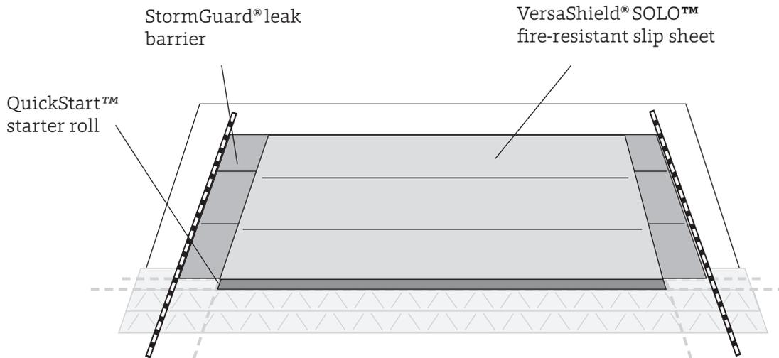
**Figure 22. Install VersaShield® SOLO Fire-Resistant Slip Sheet over field of the array**
