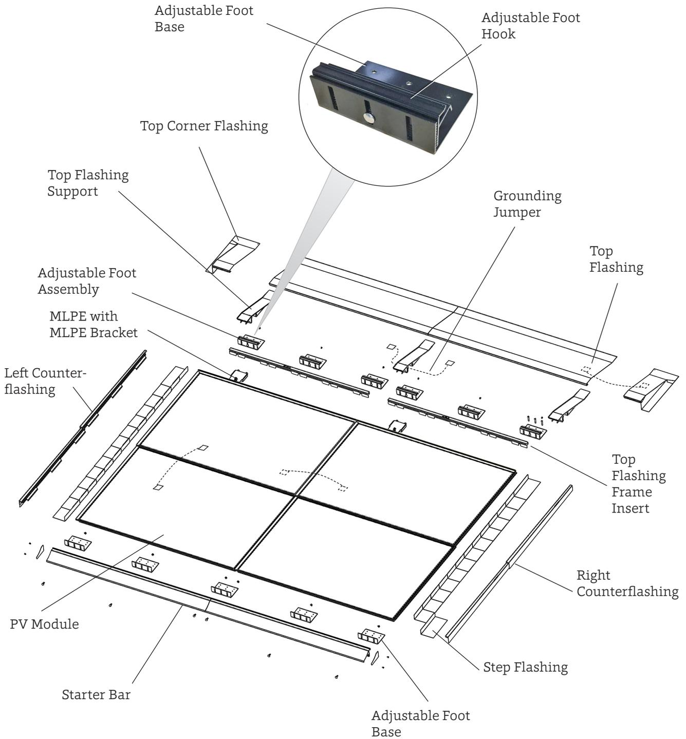
**Figure 5. GAF Energy Solar System Hardware Components**
