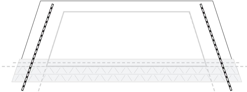
**Figure 19. Mark 3 feet out from left and right edges of array**
