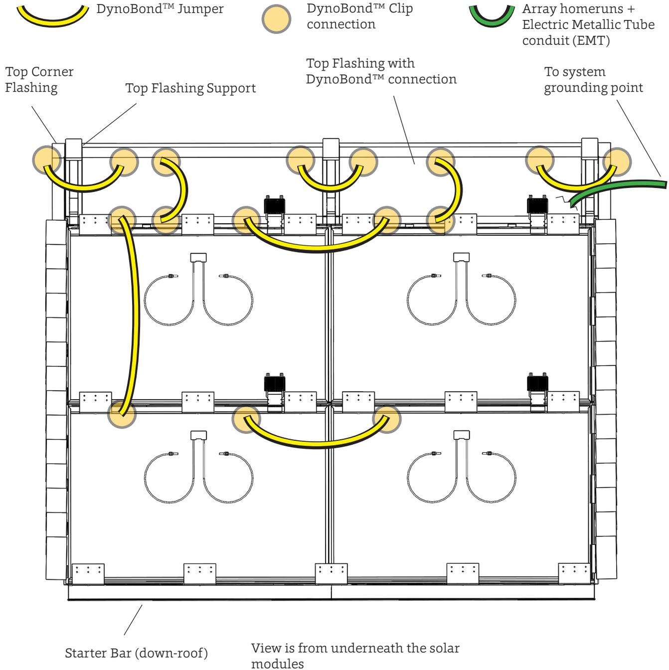
**Figure 6. GAF Energy Solar System grounding requirements**
