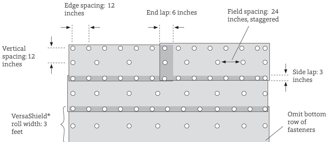
**Figure 24. VersaShield® fastener spacing and overlap, slope 4:12 - 6:12**
