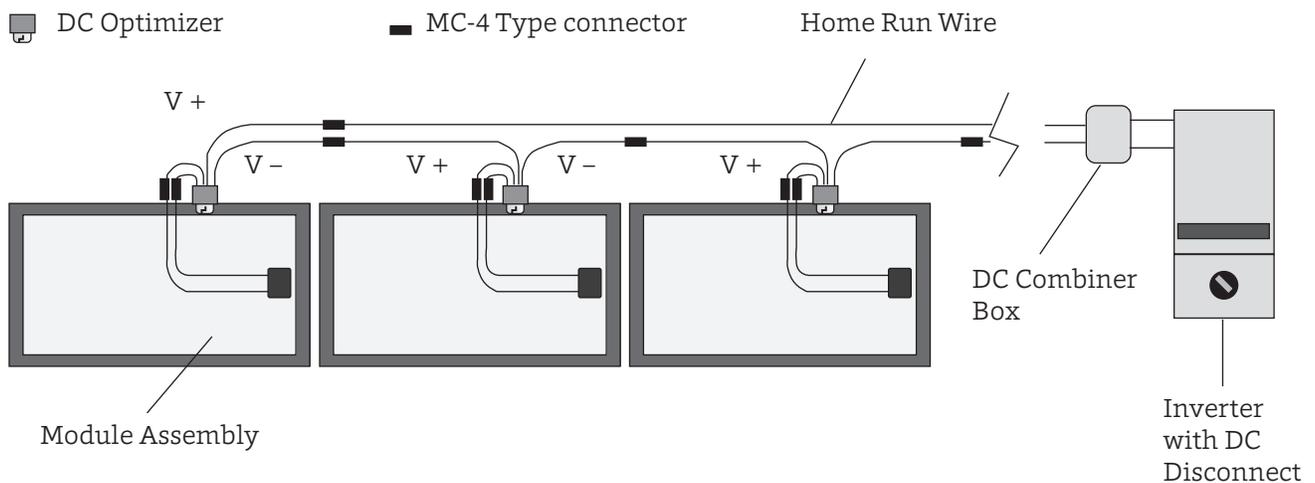
**Figure 71. Typical DC Optimizer Wiring**
