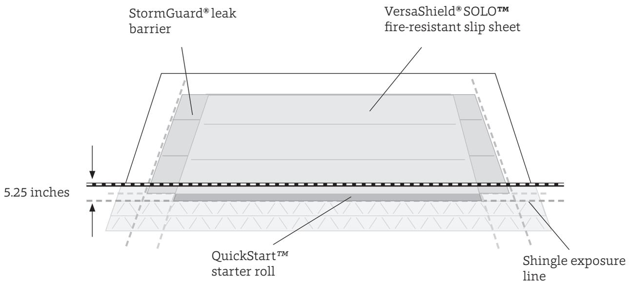
**Figure 36. Snap chalk line for Starter Bar Foot positioning**
