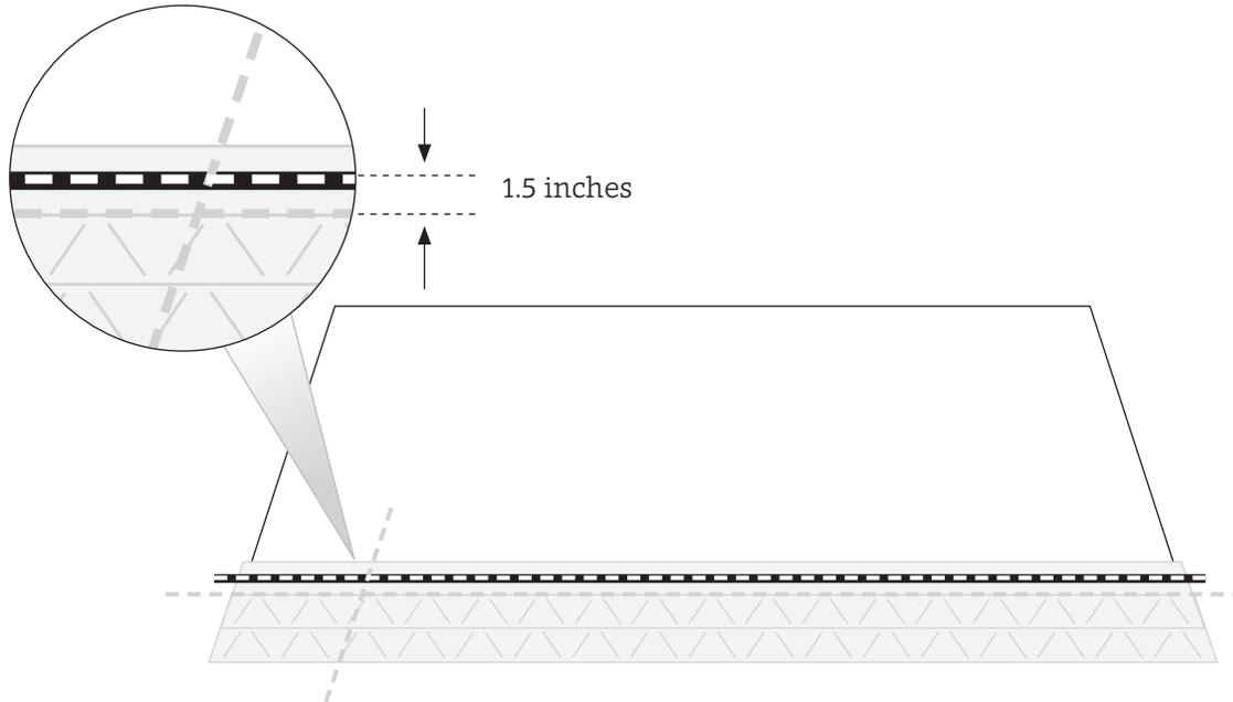
**Figure 17. Mark 1.5 inches above shingle exposure line**
