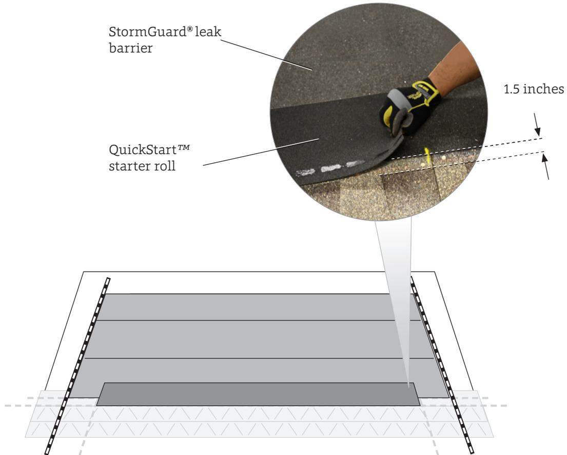
**Figure 21. Install QuickStart® Peel & Stick Starter Roll at bottom of array**
