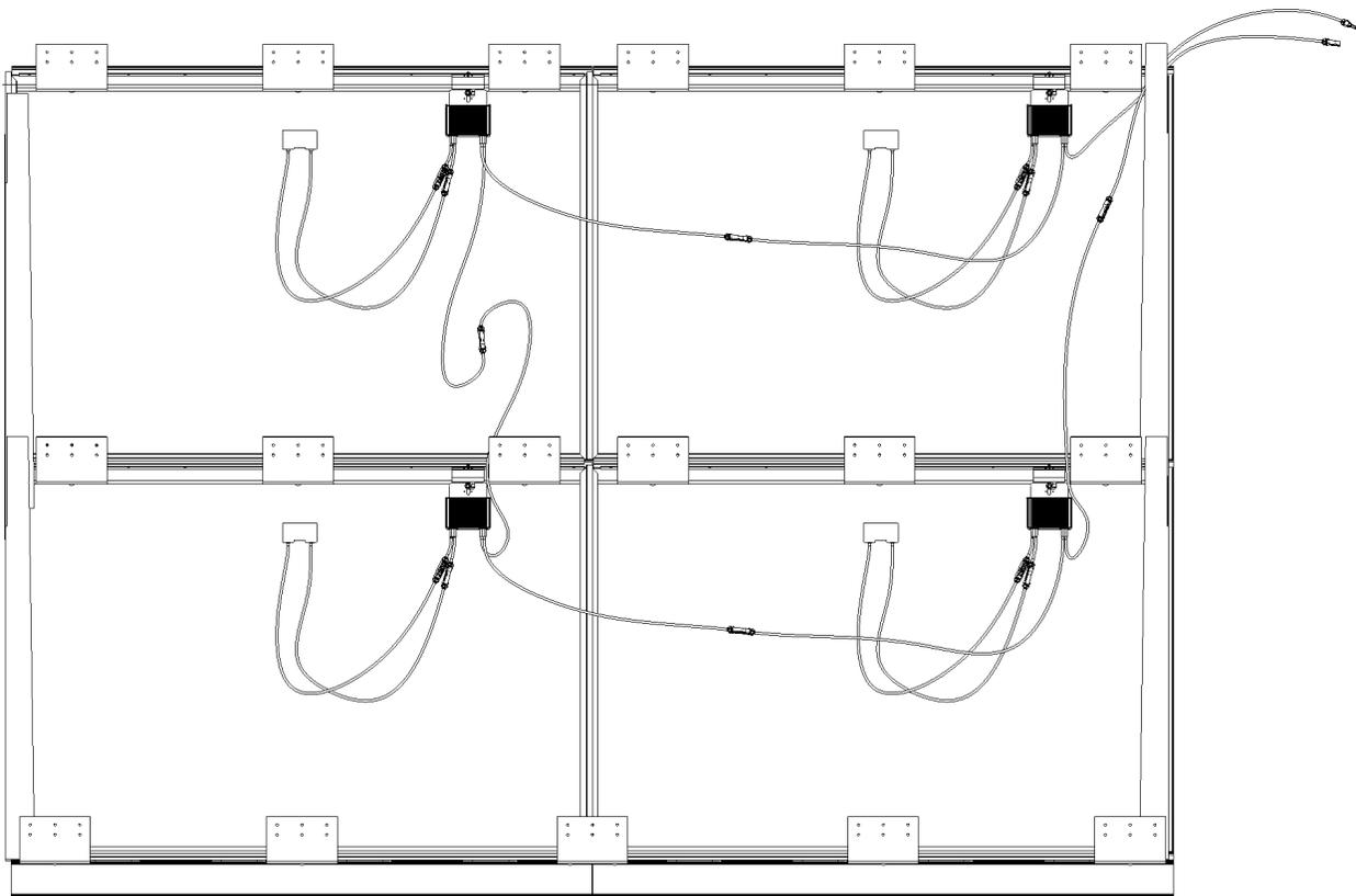
**Figure 73. Physical wire management diagram**
