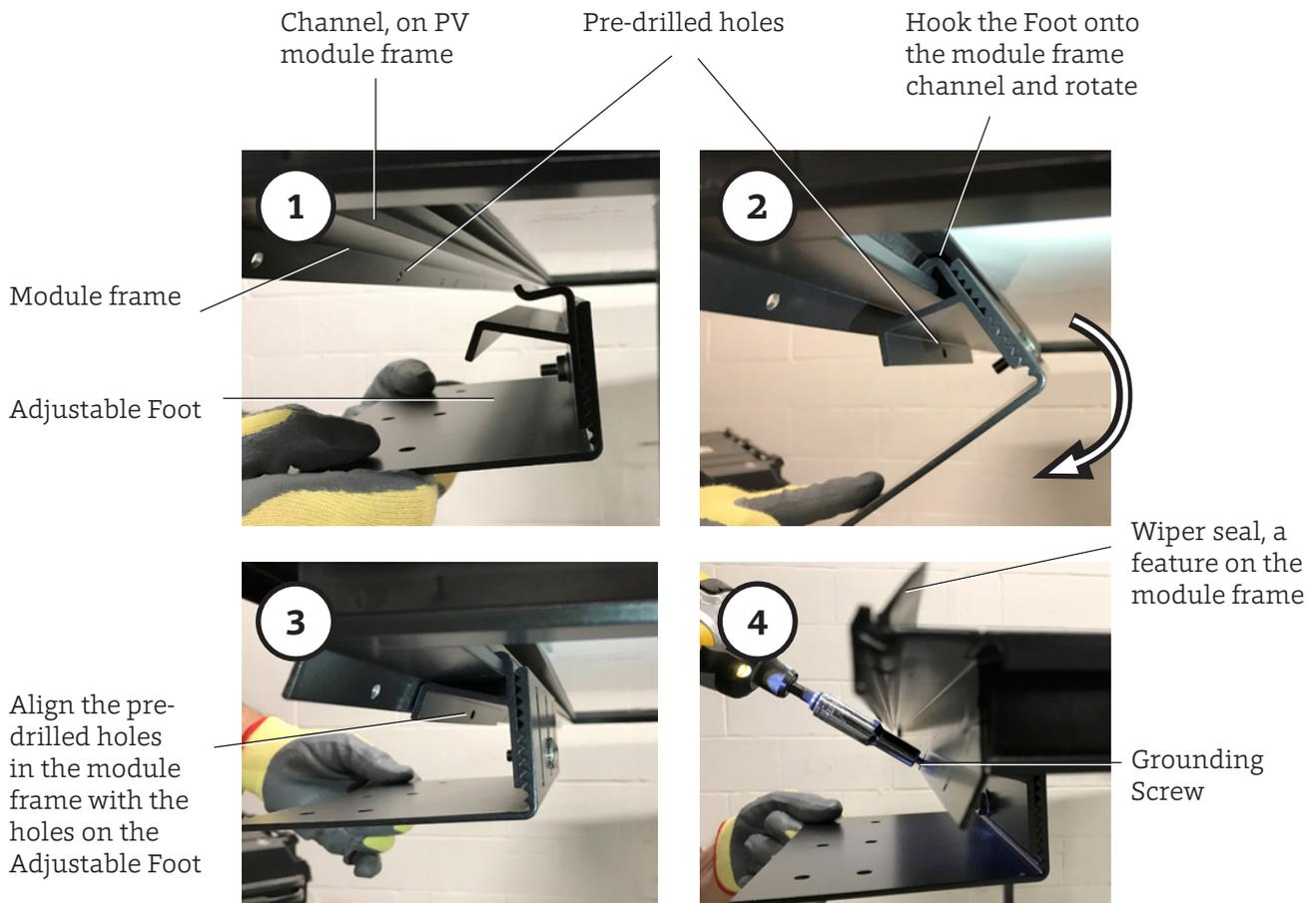
**Figure 28. Mounting the Adjustable Feet onto the module frame**
