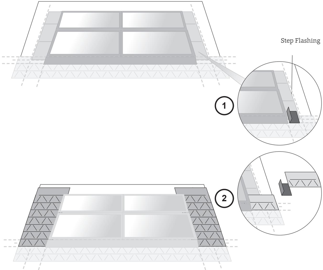
**Figure 52. Step Flashing installation sequence**
