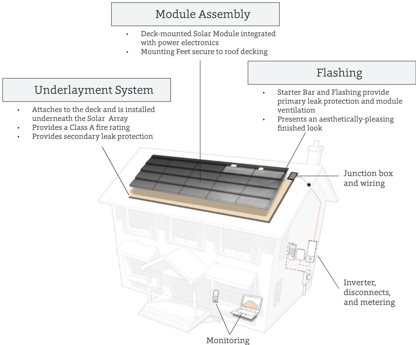
**Figure 4. Main components of GAF Energy Solar System installation**
