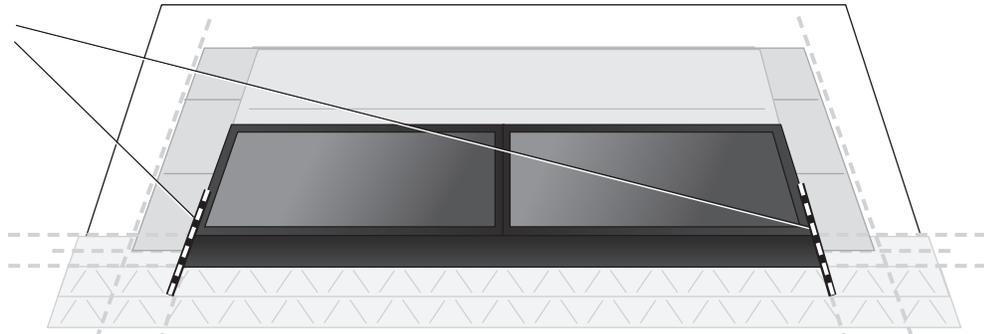
**Figure 47. Align array at both sides before securing modules to deck**
