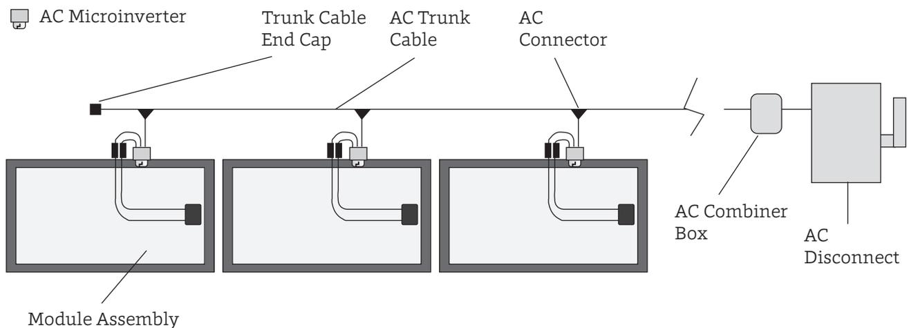
**Figure 72. Typical AC Microinverter Wiring**
